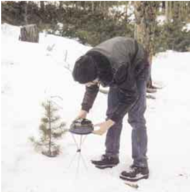
Rob's son, Abel uses a Solar Pathfinder to pick the best location for the PV panels.
